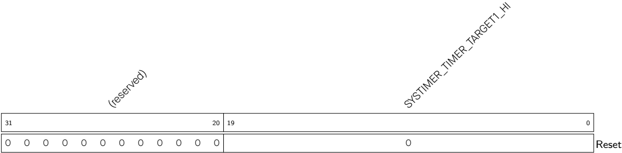
Register 10.18. SYSTIMER_TARGET1_HI_REG (0x0024)
