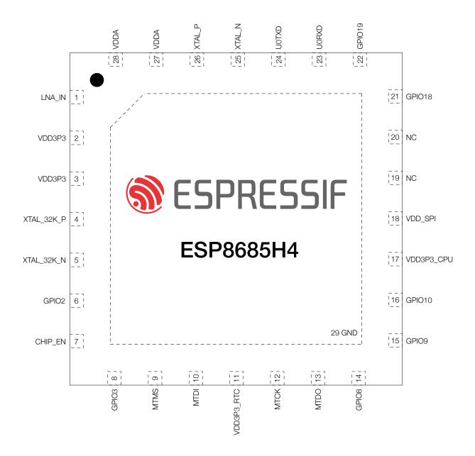
Figure 1-1. ESP8685 Pin Layout (Top View)
