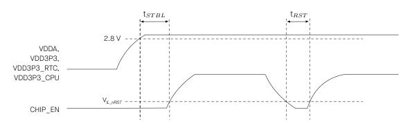
Figure 1-3. Visualization of Timing Parameters for Power-up and Reset
