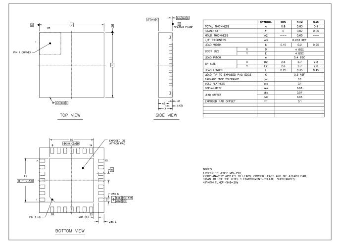
Figure 6-1. QFN28 (4×4 mm) Package
