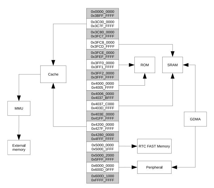
Figure 3-1. Address Mapping Structure
