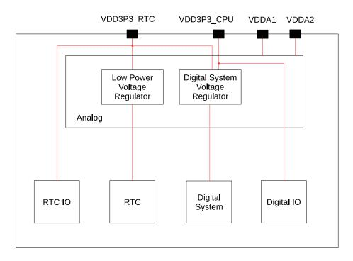
Figure 1-2. ESP8685 Power Scheme
