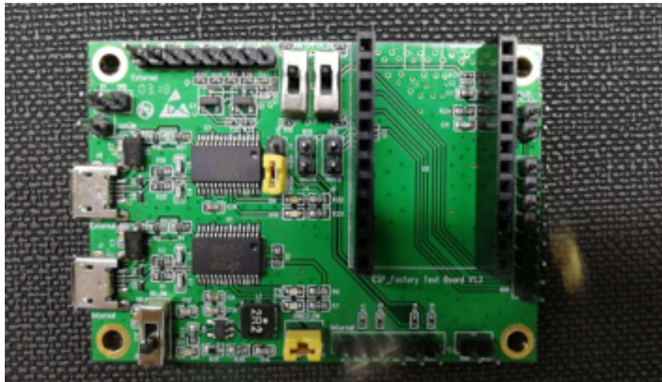
Figure 2-5. A Typical Serial Port Board (ESP\_Factory Test Board V1.3)
