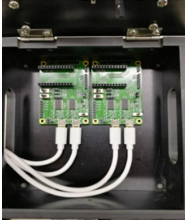
**Figure 2-6. The Placement of the Serial Port Boards in the Bottom Box**
