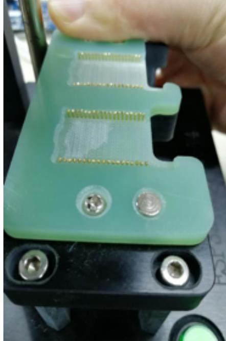
Figure 2-2. The Metal Probes (the handle is pressed)
