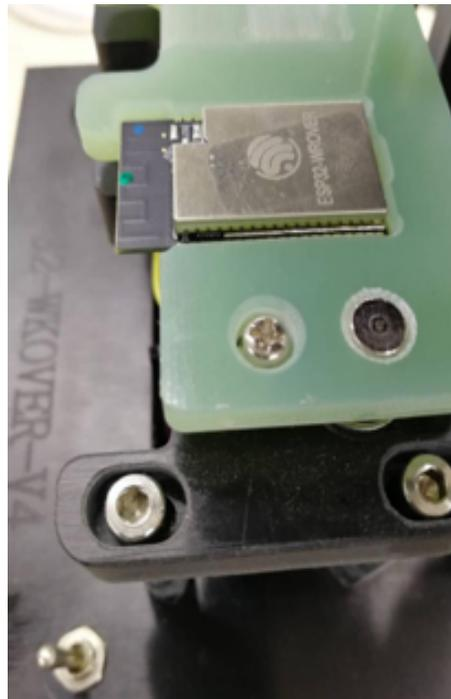
Figure 2-1. The Mounting Panel for the ESP-WROVER Test Fixture
