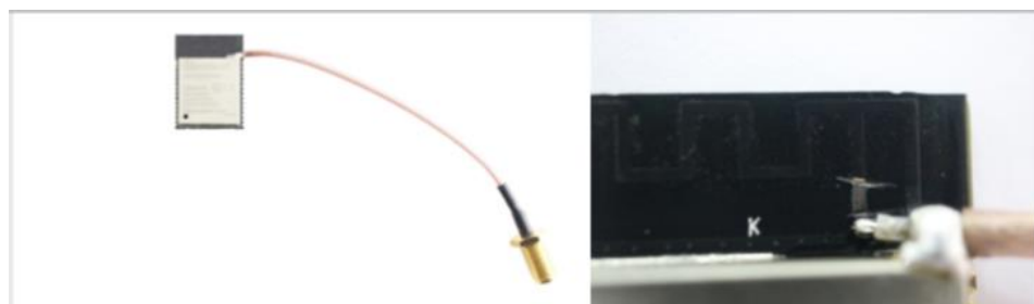
Figure 2-2. RF Cable Connection for Module Conduction Test
