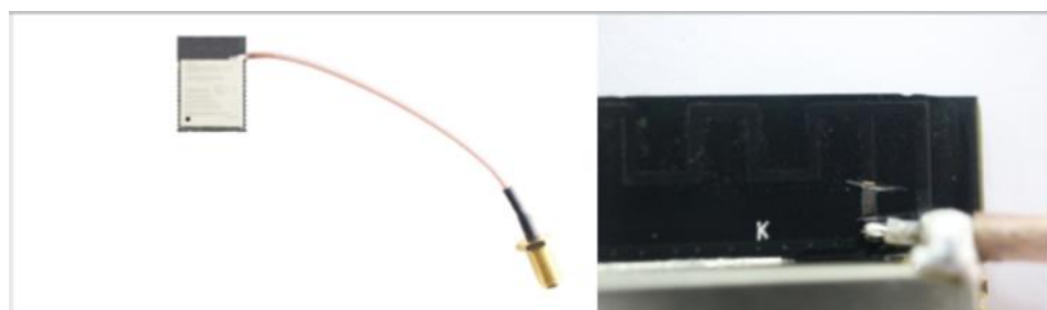
Figure 2-2. RF Cable Connection for Module Conduction Test
